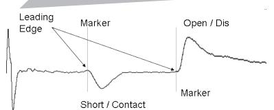
**Principle :** Time domain reflectometry, pulse reflection principles to detect impedance changes along a cable.
